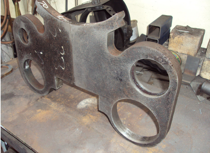
Fabricated cylinder ends , with steam passages
