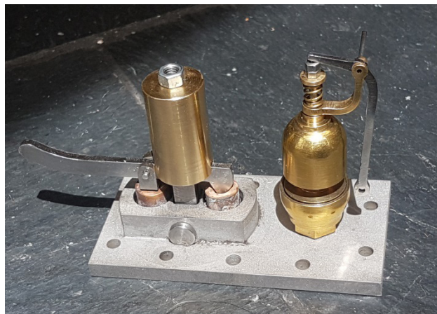
Picture shows the safety valve and whistle on the cylinder top cover.
